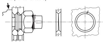
Double-capnut wheel mounting preload is force applied to the disc by torquing nuts. Inner cap nut must be tightened before tightening outer nut.
